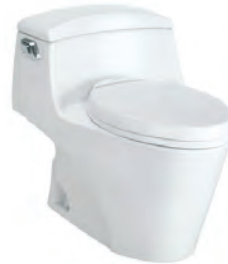
CW923GB One Piece Toilet Flush System : Tornado (4.8L) Bowl Shape : Elongated Rough-in : 305mm 510W x 720D x 665H mm
