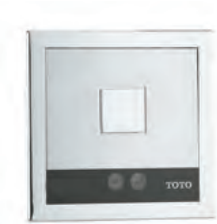
TEA99V100 (AC 220V Operated) Concealed Urinal Sensor Flush Valve w/ Manual Actuation Flush Volume : 1.5L 130W x 5D x 130H mm
