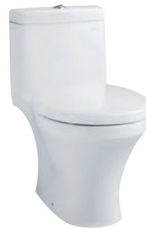
CW630JW/ F One Piece Toilet Flush System : Wash Down (4.5/ 3L) Bowl Shape : Elongated Rough-in : 220mm (S-Trap) 374W x 690D x 705H mm
