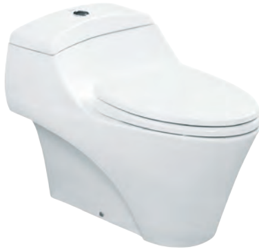
CW823NJ One Piece Toilet Flush System : Wash Down (4.5L) Bowl Shape : Elongated Rough-in : 305mm 500W x 735D x 595H mm
