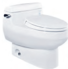
MS688V One Piece Toilet Flush System : Tornado (6L) Bowl Shape : Elongated Rough-in : 305mm 500W x 760D x 590H mm
