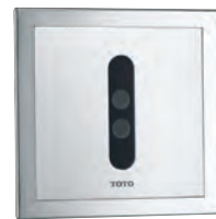
DUE111UPK (Battery Operated) DUE111UPE (AC 220V Operated) Concealed Urinal Sensor Flush Valve Flush Volume : 0.5L 130W x 5D x 130H mm
