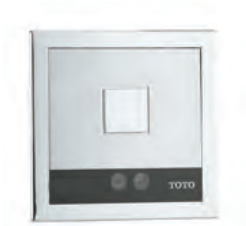
TEA99V100 (AC 220V Operated) Concealed Urinal Sensor Flush Valve w/ Manual Actuation Flush Volume : 1.5L 130W x 5D x 130H mm
