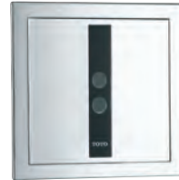
DUE111UK (Battery Operated) DUE111UE (AC 220V Operated) Concealed Urinal Sensor Flush Valve Flush Volume : 0.5L 130W x 5D x 130H mm
