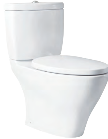
CST940 Close Coupled Toilet Flush System : Wash Down (6/3L) Bowl Shape : Elongated Rough-in : 305mm 400W x 690D x 770H mm
